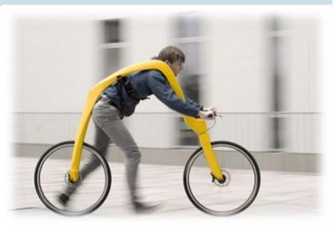
that the laminated, carbon-fiber frame and 'five-point belt system' actually makes the FLIZ more comfortable and ergonomically sound to ride as compared to traditional bicycles.
