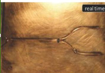
Researchers in Aalto University in Finland have developed a new concept for computing, using water droplets as bits of digital information. This was enabled by the discovery that upon collision with each other on a highly water-repellent surface, two water droplets rebound like billiard balls.
